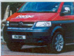
2010 Modified T5 Forge Motorsport's T5 Workhorse 130 bhp LWB van now runs at 175 bhp.
